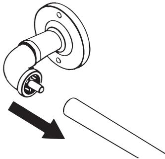
5. Attach Rod by Turning Clockwise into Bracket
