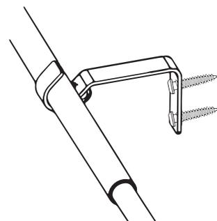
3b. Install Screws for Ceiling Mount
